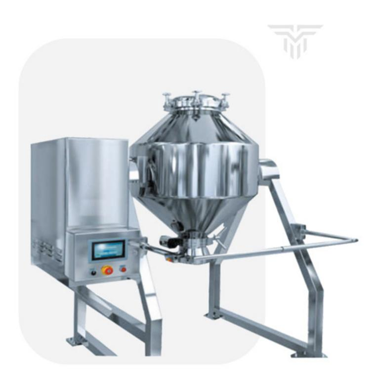
All the contact parts are made of stainless steel. The effective volume for optimum homogeneity is between 35-70% of gross volume. The SLANT double cone design eliminates dead sports, which occasionally occur in conventional double cone mixer. It can be used for pharmaceutical, food, chemical and cosmetic products etc.
